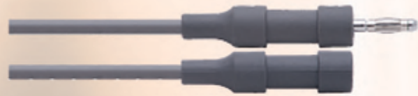
Silicone Monopolar Endoscopic Cable 10" (3.0m) SI 19.250 Instrument Connector: 4.0mm Female Plug Generator Connector: Standard 4.0mm Banana Plug Compatibility: Valleylab, Conmed & All ES Generators
